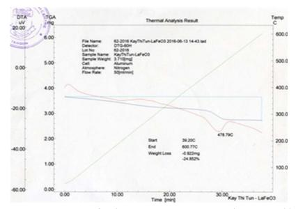
**Figure 2:** TG-DTA curve for the precursor LaFeO<sub>3</sub> powder prepared by co-precipitation method
