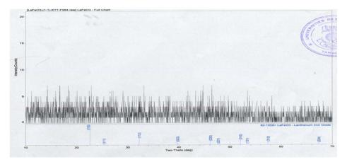
**Figure 3:** XRD diffraction pattern of xerogel LaFeO<sub>3</sub> powder obtained by citrate sol-gel method
