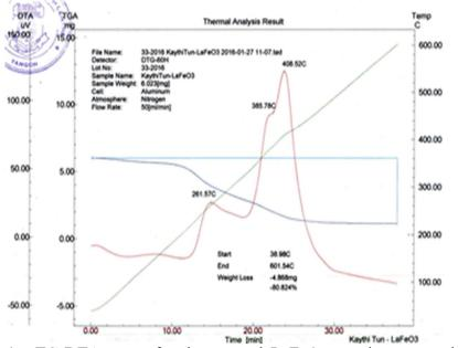
**Figure 1:** TG-DTA curve for the xerogel LaFeO<sub>3</sub> powder prepared by citrate sol-gel method
