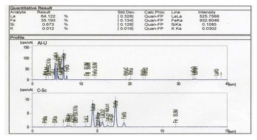
**Figure 9:** EDXRF spectrum of LaFeO<sub>3</sub> nanopowder synthesized by citrate sol-gel method calcined at 450°C for 4 h
