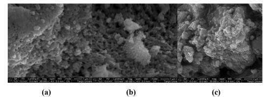
**Figure 11**: SEM micrographs of LaFeO<sub>3</sub> nanopowder prepared by citrate sol-gel method calcined at (a) 400°C (b) 450°C (c) 500°C for 4 h
