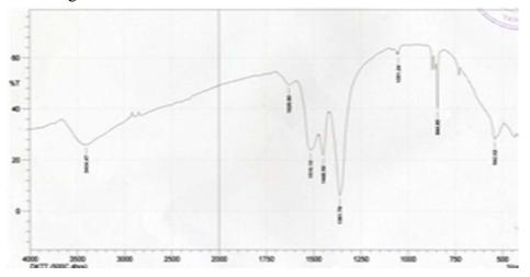
**Figure 8:** FT IR spectrum of LaFeO<sub>3</sub> nanopowder prepared co-precipitation method calcined at 500°C for 4 hours
