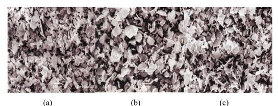
Figure 12. SEM micrographs of LaFeO<sub>3</sub> nanopowder prepared by co-precipitat method at (a)500 °C (b) 550 °C and (c) 600 °C for 4 hours
